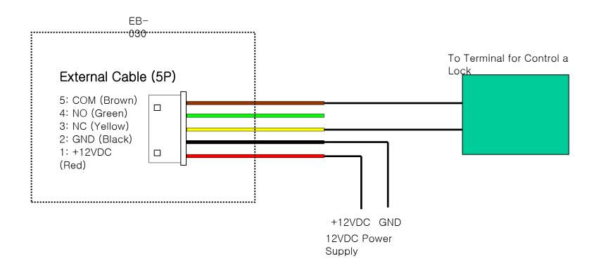
\* You must supply +12VDC Power to the terminal after completing the installation of the EB-030 because of touch-sensitive type specification. Otherwise, it may not operate properly.
