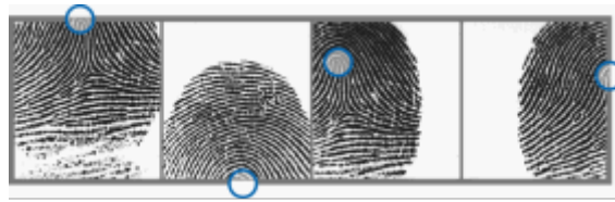
Finger 4 [ Improper Fingerprint Core Position ]
