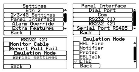
This setting can also be made using AT command AT%A14=18.
